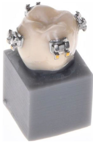
Fig. 2 One of the crowns included in the study with one metal bracket bonded to each of the four buccal surfaces
